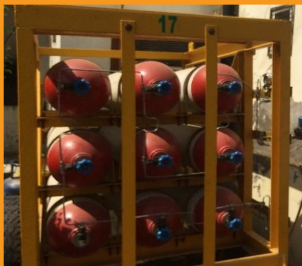
Arc Bio Fuel bio-CNG cylinder cascade
